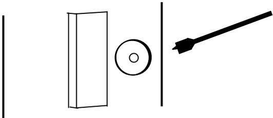
**2** Mount base plate in hole using long screws, pre-drill as necessary
